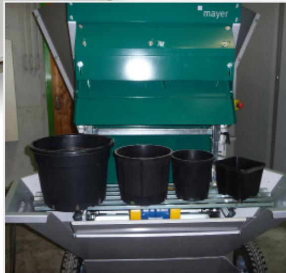
**The TM-2018 is a fast, reliable, and efficient potting machine for filling either round or square containers as well as poly bags without a drilling system.**
